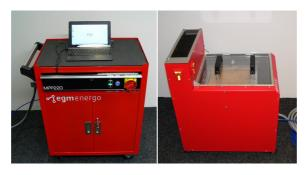
MPP-220 is a special measurement device used for measurement of thermal and water-vapour resistance under steady-state conditions ("sweating guarded-hotplate test") of textiles according to ISO 11092.
