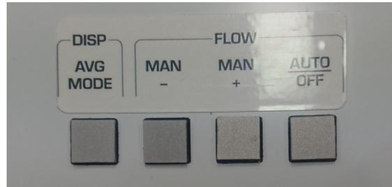
fig. 3.3: Control Panel Buttons
