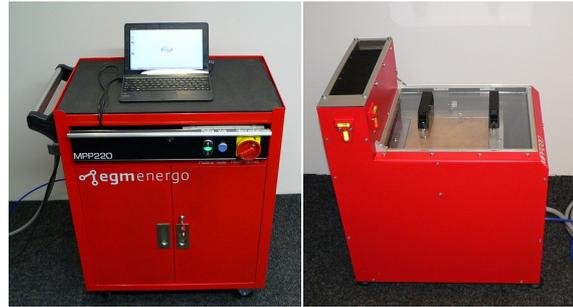
MPP-220 is a special measurement device used for measurement of thermal and water-vapour resistance under steady-state conditions („sweating guarded-hotplate test“) of textiles according to ISO 11092.
